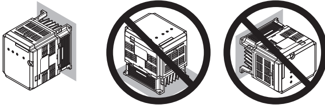
Figure 7 Correct Installation Orientation (Braking Unit)
